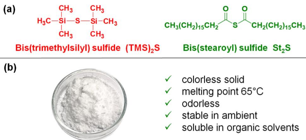
Figure 1. (a) Molecular structure of the sulfur precursors used in this work (a) and appearance and material properties of St 2 S.
