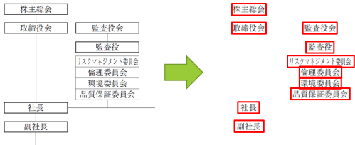
Fig. 10. Step 9: Detecting textboxes in the original PDF and recording their content, position and size.
