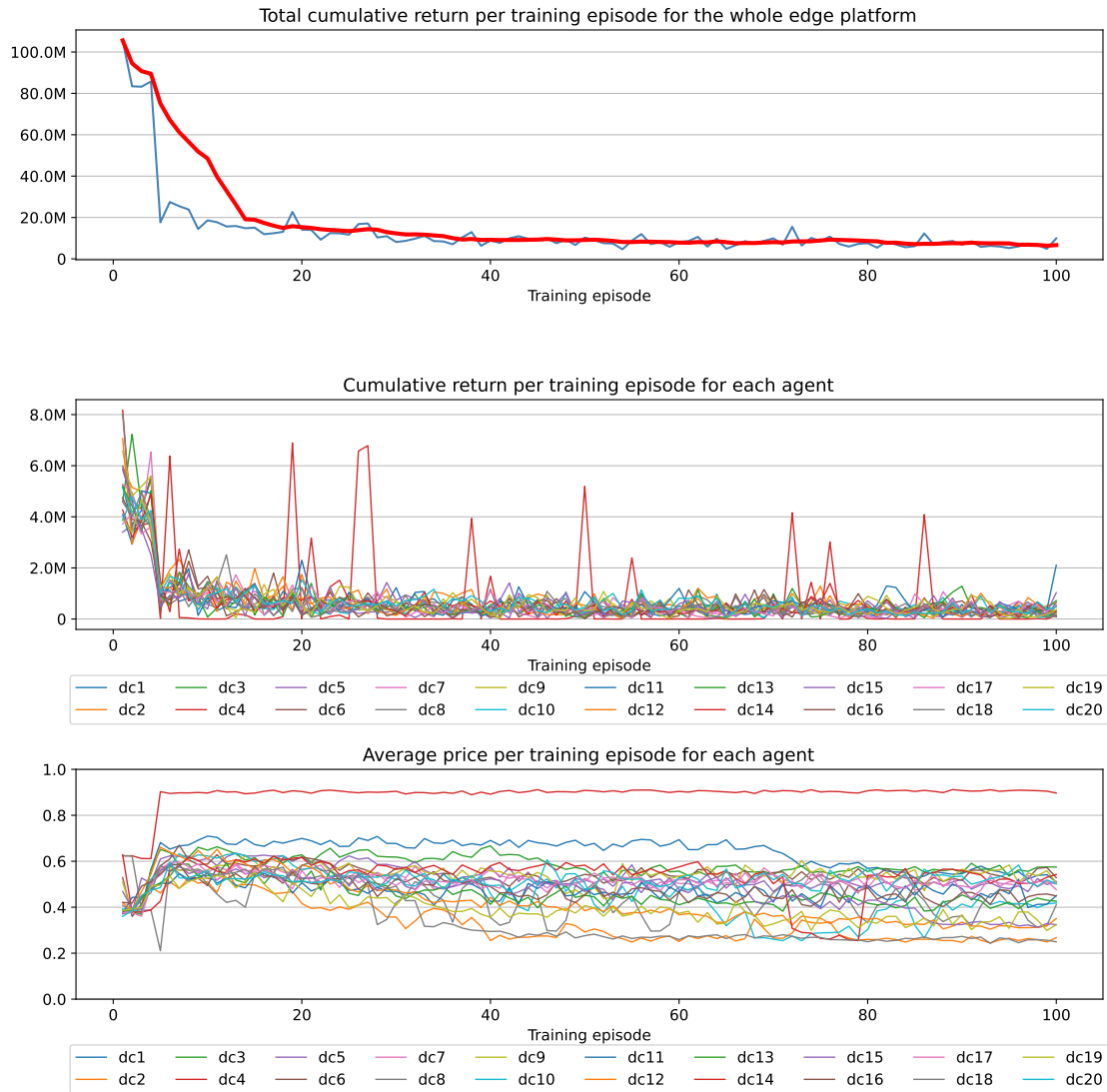
Figure 5: An example of a training plot. The training progress is shown for the decentralized control topology scenario with 20 edge servers and 2000 mobile users.
