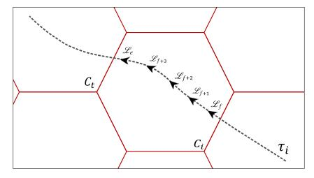
Figure 7: An example of AIS coordinates  $\mathcal{L}_f$  first and  $\mathcal{L}_e$  last of a vessel inside a grid cell  $C_i$  (current) and  $C_t$  (subsequent) on the vessel trajectory  $\tau_i$ .
