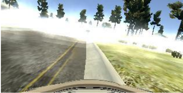
Fig. 4. Dave-2 simulation out of bounds caused by fog
