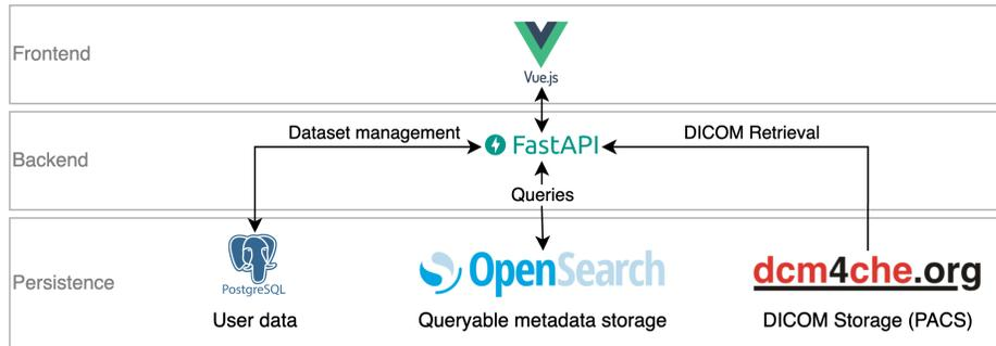
**Fig. 2.** Illustrating the technical infrastructure. Highlighting the frontend powered by Vue.js, the backend using FastAPI, and the three-fold data persistence layer consisting of dcm4chee, OpenSearch, and PostgreSQL. The arrows visualize the communication between the components.
