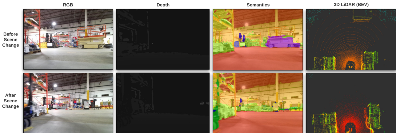
Fig. 4: A sample RGBD, semantically labelled, and 3D LiDAR frame captured by the sensors before ( top ) and after ( bottom ) the scene changes. The forklift in the top frame, captured June 15, 2022, is no longer present in the bottom frame, captured Oct. 23, 2022.
