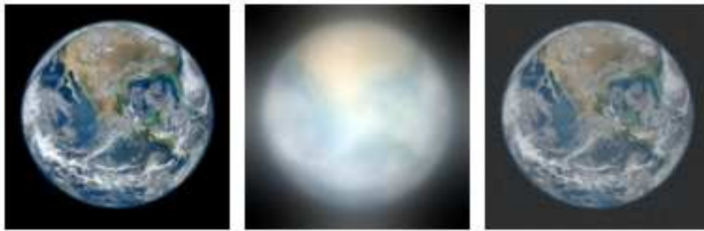
FIG. 12: Imaging simulation with the SGL. Left: original RGB color image of an Earth-like exoplanet with 1024 \times 1024 pixels; center: image blurred by the SGL, sampled at an SNR of \sim 10^3 per color channel, or overall SNR of 3 \times 10^3 ; right: image deconvolution result (see [115, 116] for details).
