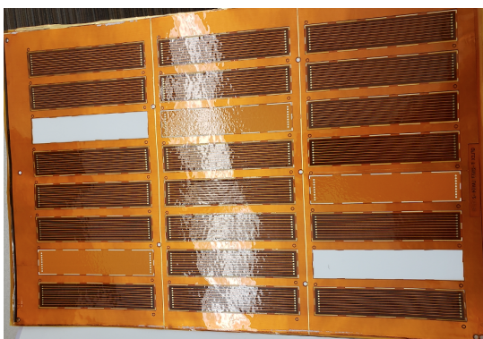
Figure 2: An example of a panel of detachable coupons with typical cable features, utilized to study the contamination levels at each step of the fabrication process.
