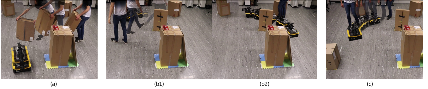
Fig. 5: (a): We dynamically put an obstacle in the trajectory of the robot which causes it to stop. The robot then waits until the obstacle is removed and continues its trajectory. (b1, b2): Dynamic interactions with the robot by first walking next to it (b1), then overtaking it and standing to the side of the box (b2). While the person walks next to it the robot continues its trajectory. When the person overtook the robot, it swings to the right to avoid the collision. (c): The person walks towards the robot. To avoid the collision, the robot drives backwards. The complete video is available at https://youtu.be/gAcETwOWTM4 .
