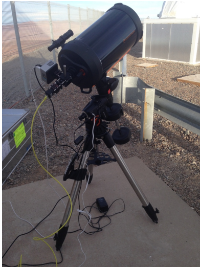
Figure 1. The SHIMM (with additional FASS optics) at Cerro Paranal, Chile, at the site of the VLT (Guesalaga et al. 2016).
