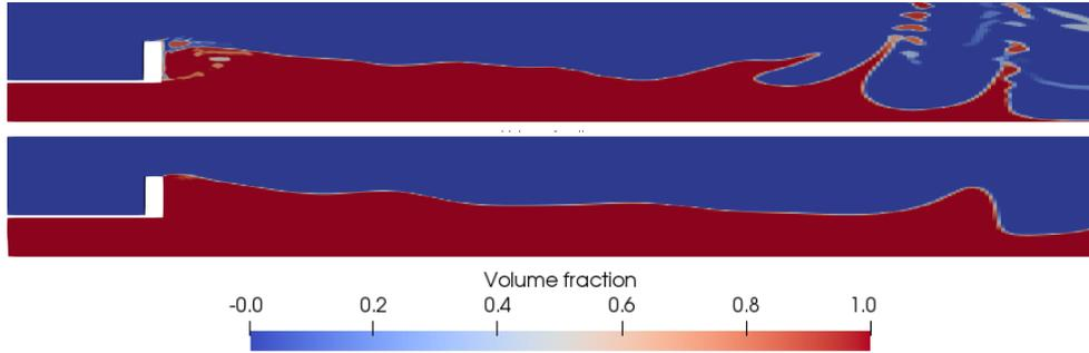
Figure 9: Volume fraction  $\alpha$  shows the difference in atomization and interaction when not including surface tension (top) or when including it (bottom).
