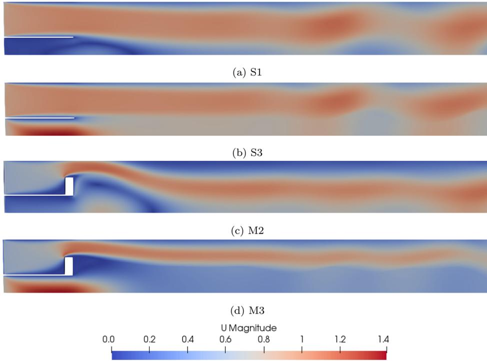
Figure 7: Velocity magnitude at a representative instant once the permanent stage has been reached for four different multiphase cases.
