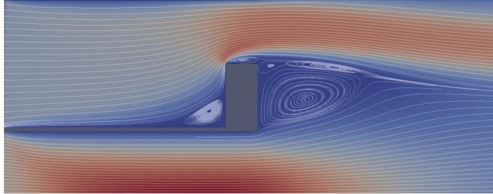
Figure 8: Streamlines around the bluff body. Colors represent velocity magnitude, where red implies large velocity magnitude and blue refers to small velocity.
