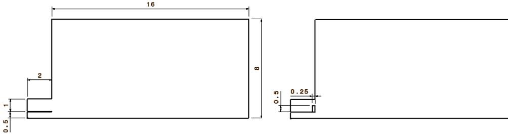
Figure 1: 2D sections of the two cases of study: Simple configuration (left) and modified configuration (right). Dimensions are specified as multiples of a characteristic length  $h$ . Notice that the bottom horizontal line corresponds to the symmetry axis of the problem.
