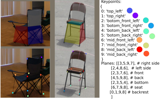
Figure 2. PPH of chair class. The planes are chosen to enclose the smallest 3D hull of the keypoints while considering the semantics of the keypoints.
