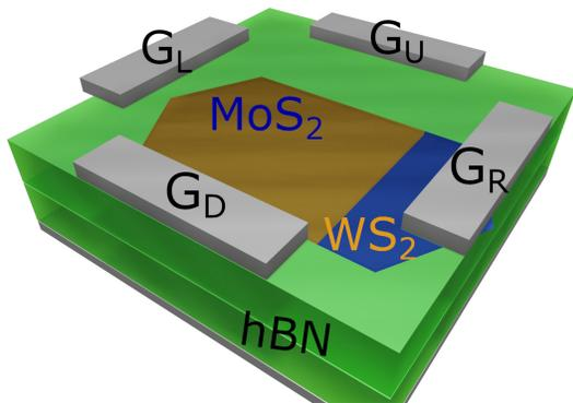
FIG. 1. The schematic view on the proposed device structure containing MoS<sub>2</sub>/WS<sub>2</sub> heterojunction (orange/blue) sandwiched between hBN tunnel barriers, together with four gates G<sub>{L,R,U,D}</sub> deposited on top defining quantum dot in the junction area.
