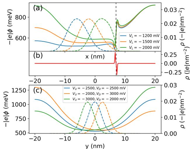
FIG. 3. (a) Potential profiles (solid lines) through the junction interface, with the characteristic CB offset built by space charge dipole (b). Modulation of top gate voltages changes the potential, also in direction along the junction (c), and shifts electron (dashed lines) confined within the QD.
