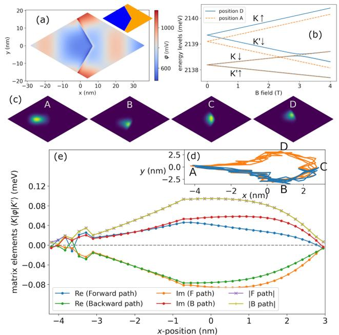
FIG. 10. Setup designed for testing a possibility of valley qubit manipulation via geometric phase accumulation. It is based on corner-shaped junction (a) with both terminations of armchair type, while the phase accumulation occurs when circulating on a closed loop (d) near the junction.
