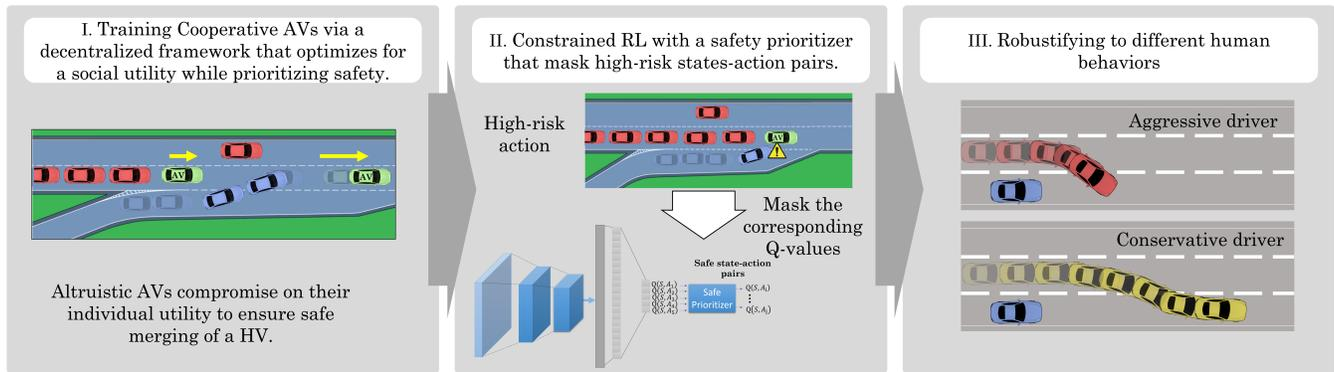
Fig. 1: An overview of our methodology for ensuring the safety and robustness of cooperative autonomous vehicles in interaction with human-driven vehicles.
