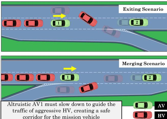
Fig. 2: Highway merging and exiting scenarios in mixed traffic where the road is shared by AVs (green) and aggressive HVs (red). Altruistic AVs must learn to coordinate to allow for a safe and efficient merging/exiting while also being robust to different scenarios and behaviors and ensuring safety in decision-making.
