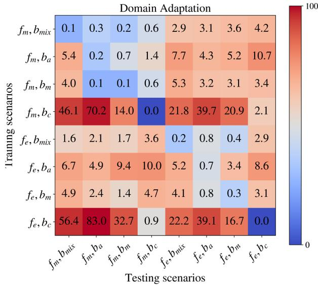
Fig. 7: The domain adaptation matrix with crash percentage ( $C(\%)$ ) between different traffic scenarios and behaviors. The lower  $C(\%)$  the most suitable the adaptability in terms of safety (measured by  $C(\%)$ ) between those domains.
