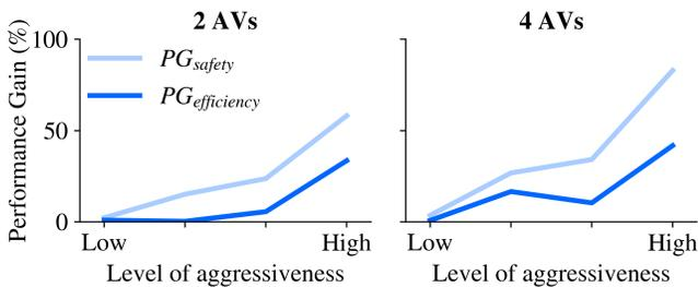
Fig. 4: Sensitivity analyses measured by altruistic performance gain (PG) of AVs, the more aggressiveness of the HVs, the higher the impact/gain of cooperation.
