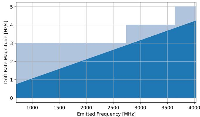
**Figure 1.** Expected Doppler drift from a transmitter located on the surface of Proxima b. Dark blue is the calculated magnitude of the Doppler drift and light blue is the magnitude of the search range.
