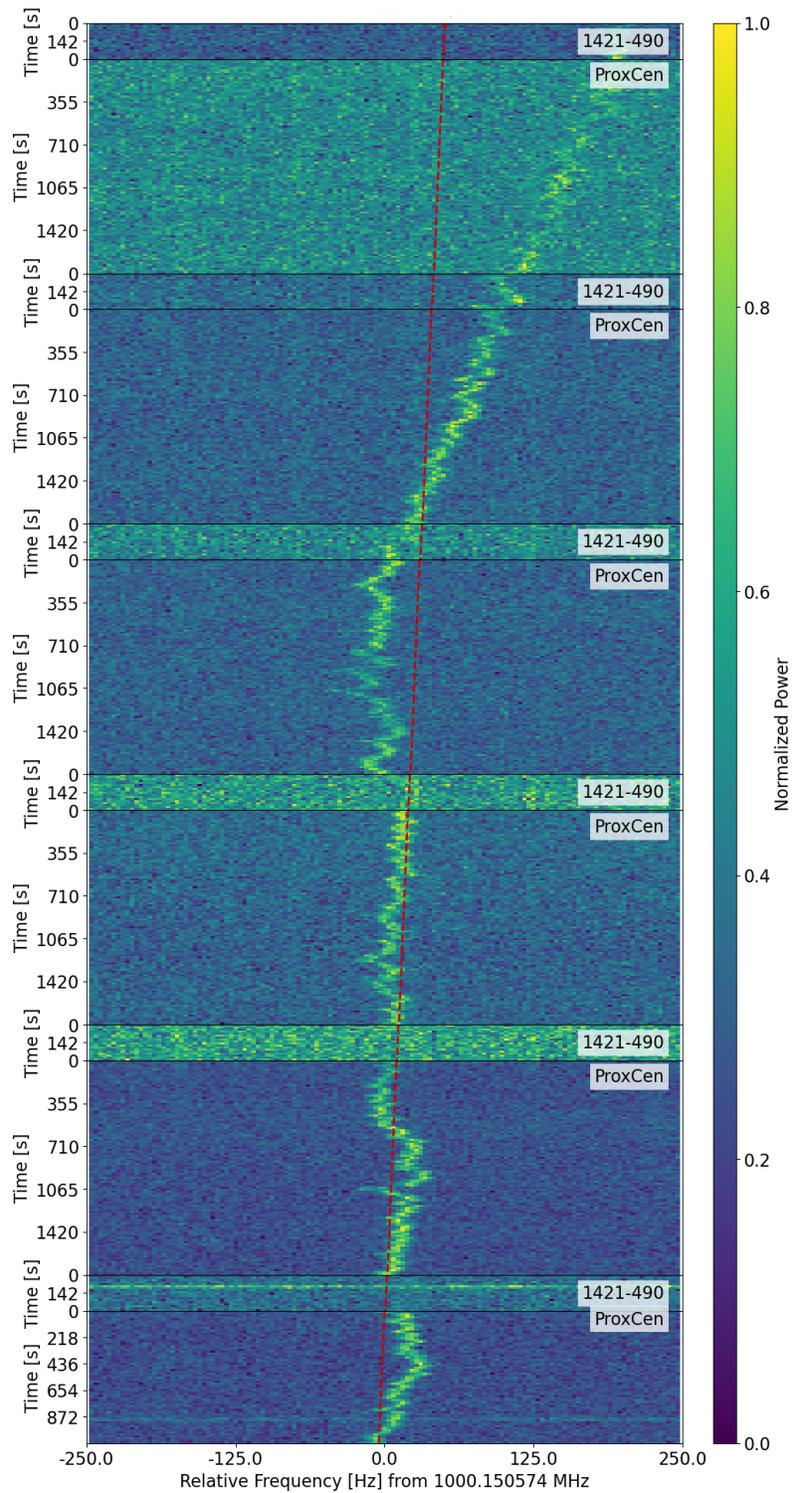
**Figure (Supplementary) 2.** An event that did not pass the second round of plotting (cadence length of 12). The signal was not visible in the off-source pointings for the first round of plotting (6th–11th pointings), but the signal is clearly visible in earlier off-source pointings that were not initially plotted.
