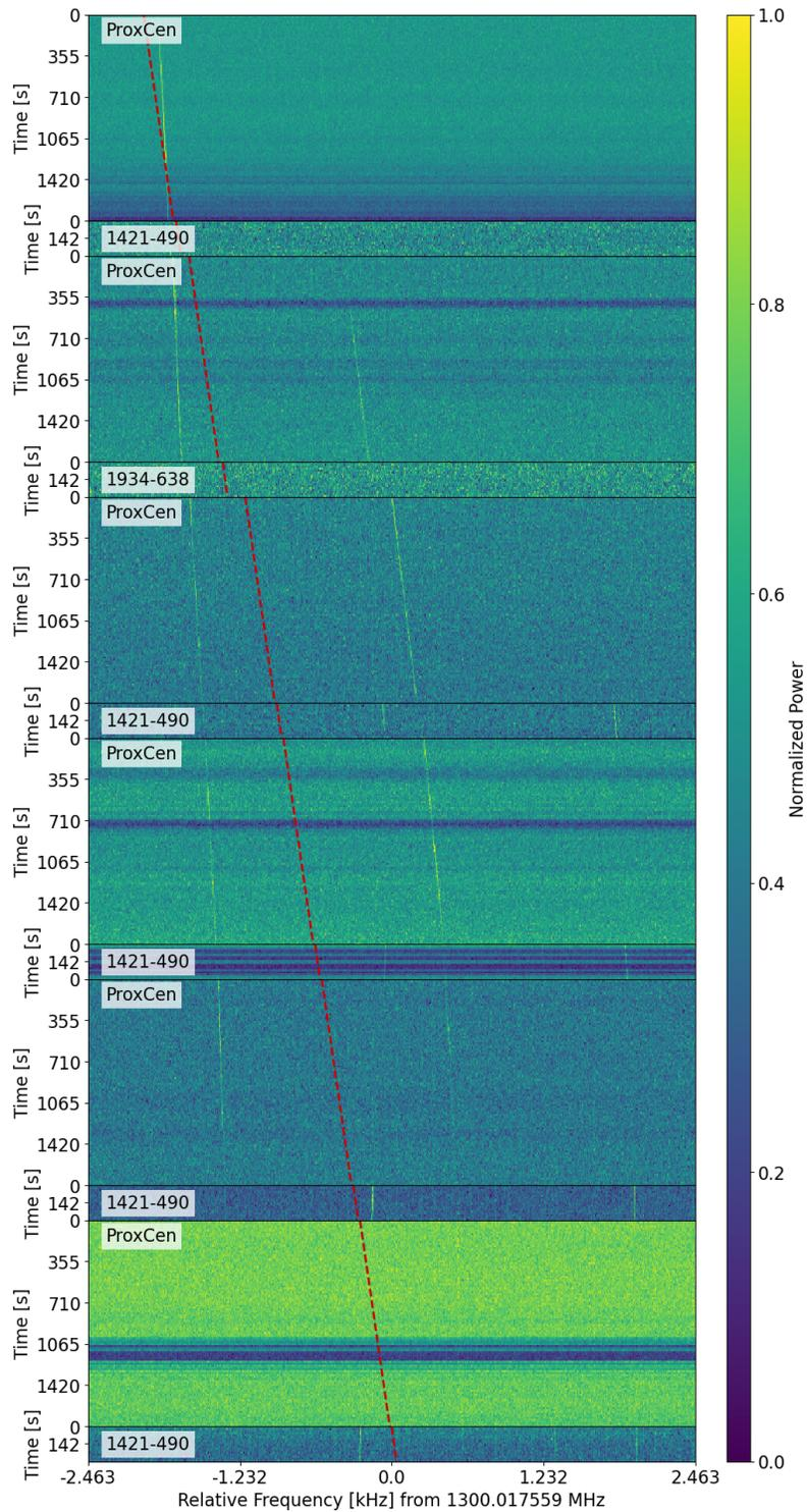
**Figure (Supplementary) 3.** Example of an event that passed two rounds of plotting, but was flagged as satellite RFI. The Global Navigation Satellite Service (GNSS) emits in the 1238 – 1318 MHz range. In addition to the two events visible in a majority of the on-source pointings, two similar events are visible in some of the off-source pointings. This is likely due to another GNSS satellite that is close to our pointing of PKS 1421-490.
