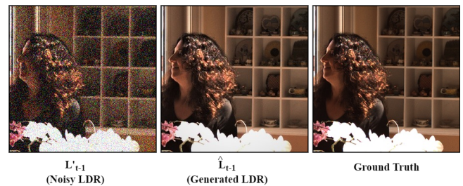
Figure 8: Visual comparison of a reconstructed clean LDR frame using denoising network from a noisy LDR frame of a scene used previously in Figure 2
