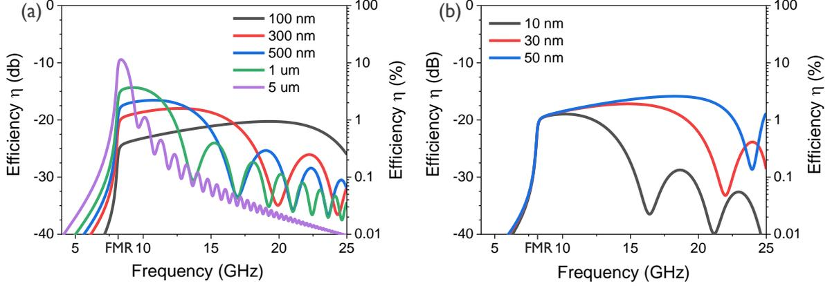
FIG. 5: Power transmission efficiency  $\eta$  into the magnetic system ( $\zeta = \frac{1}{2}$ , maximum power transfer) in the Damon–Eshbach configuration (a) as a function of the inductive antenna width  $w$  between 100 nm and 5  $\mu\text{m}$  ( $W = 1 \mu\text{m}$ ,  $t = 20 \text{ nm}$ ) and (b) as a function of waveguide thickness  $t$  between 10 nm and 50 nm ( $W = 1 \mu\text{m}$ ,  $w = 300 \text{ nm}$ ). The FMR frequency at 8.1 GHz is indicated in both graphs as a reference.
