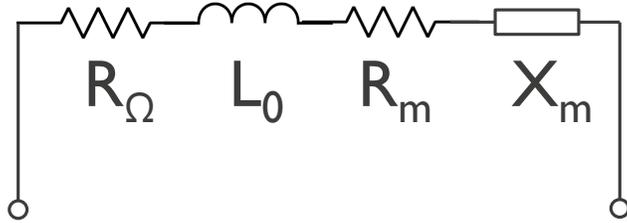
FIG. 1: Lumped equivalent circuit representation of an inductive antenna spin-wave transducer. The equivalent circuit consists of an Ohmic series resistance ( $R_\Omega$ ), a self-inductance ( $L_0$ ), as well as a radiation resistance ( $R_m$ ) and reactance ( $X_m$ ) that capture the power coupling to FMR or spin waves.
