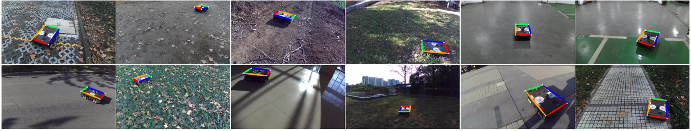
Fig. 10. Visualization of the keypoints detection. Different types of keypoints are connected by edges with different colors.
