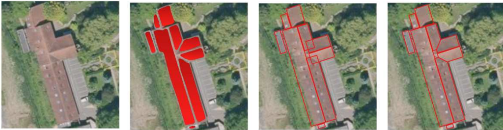
Figure 4: Illustration of the roof vectorization and regularization process. From left to right: raw aerial image, U-Net segmentation, oriented bounding boxes and fitted predictions using geometric approaches.
