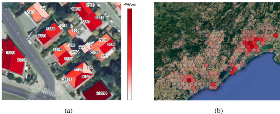
Figure 3: (a) Neighborhood view of the resulting solar potential. (b) Aggregated view (sum) of the solar potential over French Hérault department.
