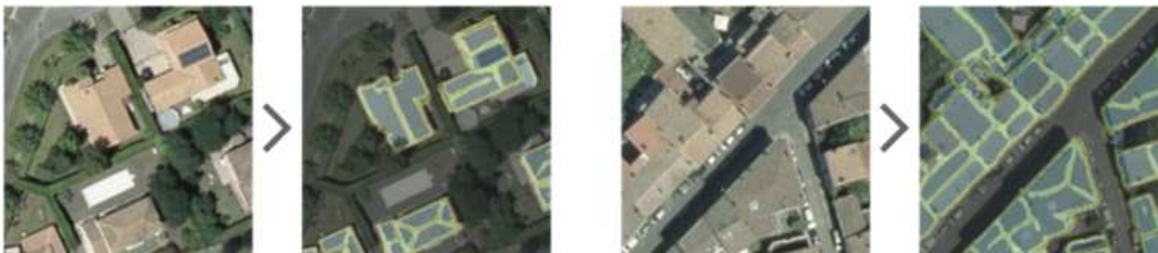
Figure 2: Two examples of aerial image and roof sections semantic segmentation pairs. Sections are depicted in blue, ridges in yellow.
