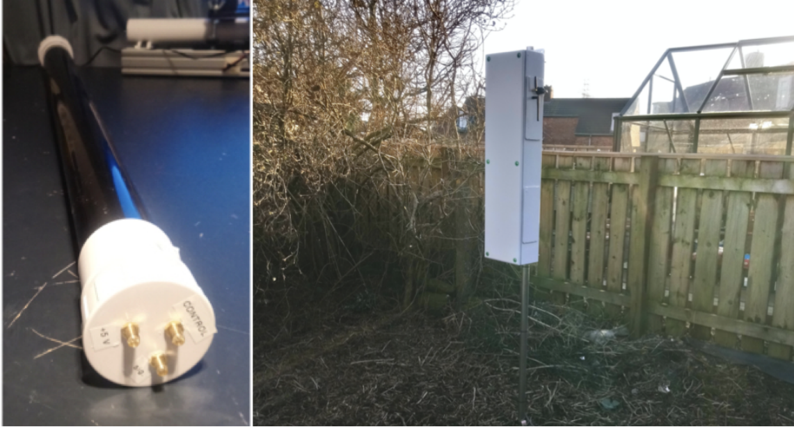
Figure 7. Assembled detector prototype. (left) Bare detector tube before being surrounded in LDPE moderator. (right) Assembled IP55 weatherproof detector system mounted onto a pole.
