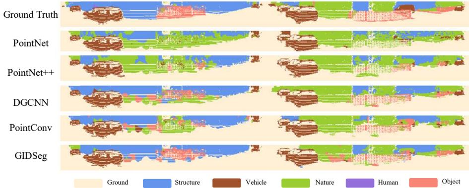
Fig. 3. **Segmentation results on *SemanticKITTI* dataset.** Spherical view projection of 3D semantic segmentation results of different point-based methods.
