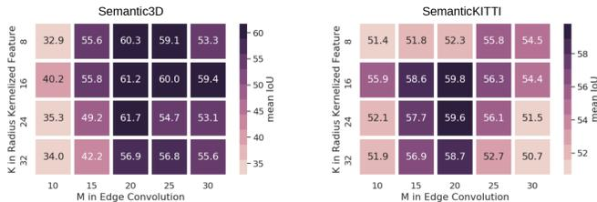
Fig. 6. **Ablation study for the radius kernel and edge convolution.** The mean IoU under different settings of  $K$  of radius kernel function and  $M$  in edge convolution layer on (a) *Semantic3D*, (b) *SemanticKITTI* dataset.
