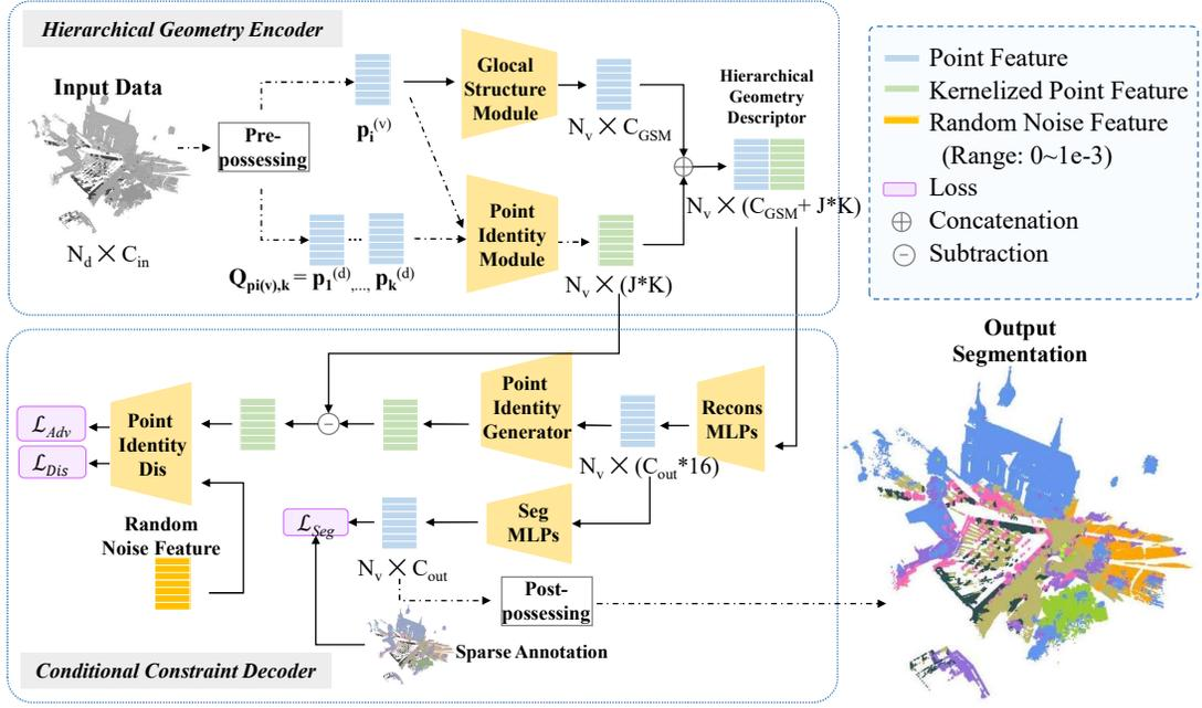
Fig. 2. **Architecture of GIDSeg for point cloud semantic segmentation.** The framework consists of a Hierarchical Geometry Encoder (HGE) for projecting the voxelized-level and dense level descriptors to a canonical space, coupled with a successive Conditional Constraint Decoder (CCD) to generate all labels for each points.
