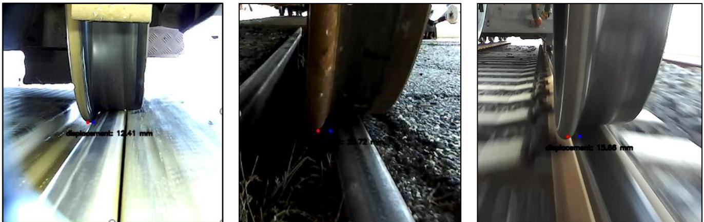
**Fig. 12.** Real-time lateral displacement measurement of the wheel on the rail to support track geometry monitoring (screenshot from the demo videos <https://youtu.be/it21cE87LCM>, <https://youtu.be/Nc1bkOdkkSM> and <https://youtu.be/K5HnUixyGxo>)
