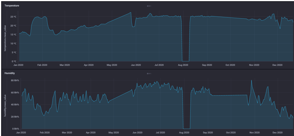
Fig. 7. Evolution of the temperature (top) and humidity (bottom) of the clean room collected by a Pi from Jan., 2020.
