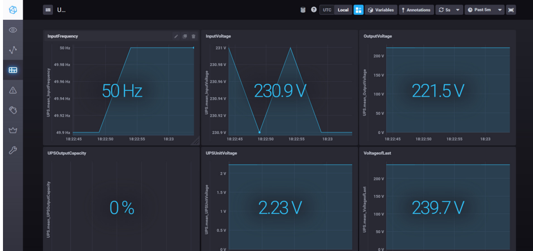
Fig. 1. Example of the custom dashboard. The dash board displays the time curve and current value of parameters of the UPS, such as the input voltage and the frequency.
