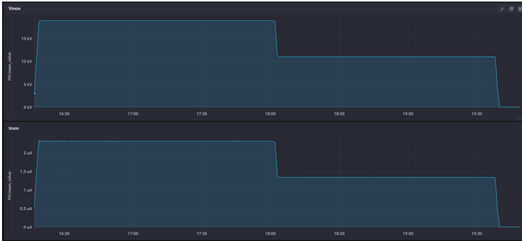
Fig. 4. Example of the voltage (top) and current (bottom) from the Matsusada AU HV power supplies during a data taking run, collected by the P-SCS.
