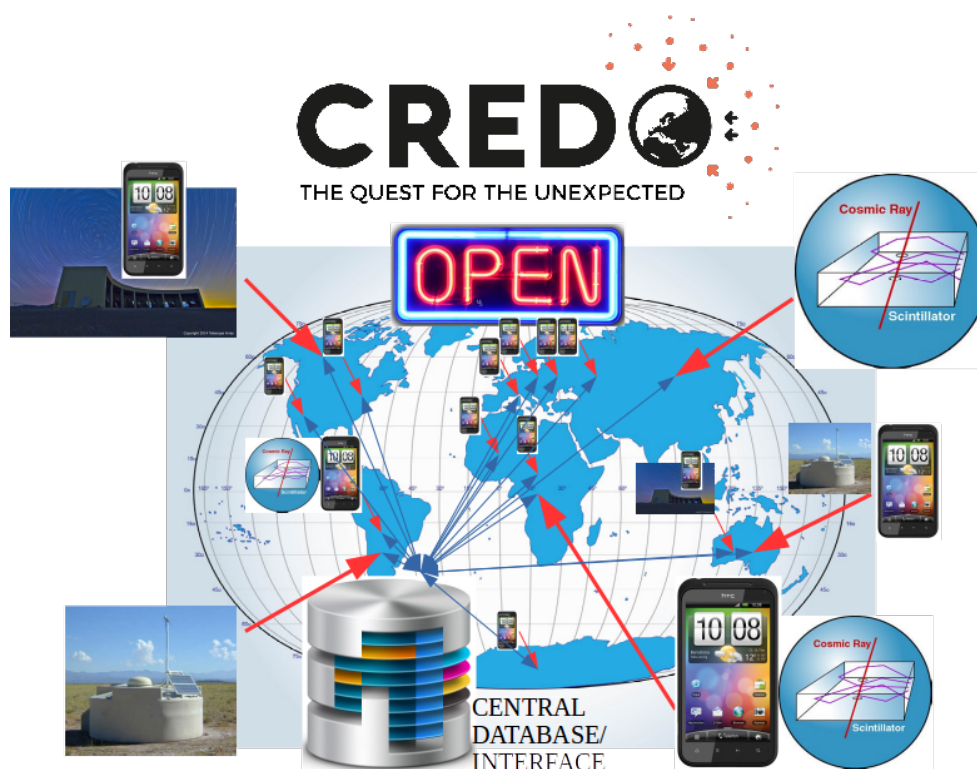
Figure 7. The concept of the Cosmic Ray Extremely Distributed Observatory (CREDO): open on two ends (data upload and access), using both professional, dedicated cosmic ray infrastructure and off-the-shelf detection solutions, including smartphones.
