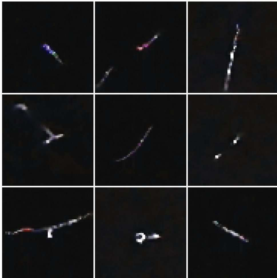
Figure 18. Example particle candidate tracks recorded with a smartphone using the CREDO Detector mobile application. [source: the CREDO Collaboration materials and measurements]
