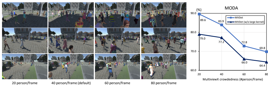
Fig. 7. MultiviewX dataset under different crowdedness configuration (left), and corresponding MVDet performance (right).
