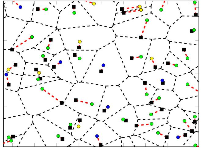
Fig. 1: A network realization for  $\lambda = 10^{-6}$  BS/KM<sup>2</sup>,  $\theta = 1$  and  $T = 8$ . Black squares depict the BSs while green, blue and yellow circles represent devices with empty queue, devices with the same  $\beta$  and devices with residual packets attempting a retransmission due to past failed attempts, respectively. The coverage region of the BSs and their connected devices are represented by dashed black and red lines, respectively.
