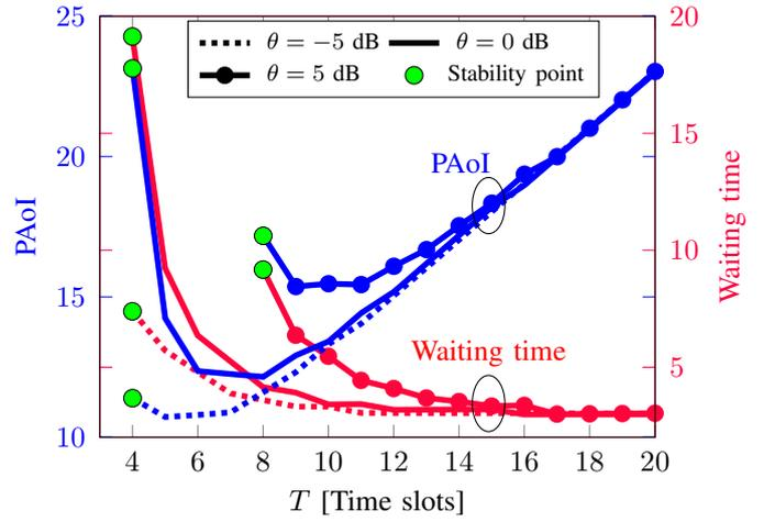
Fig. 7: PAoI (left) and average waiting time (right) for TT traffic with increasing duty cycle  $T$  and different  $\theta$ .
