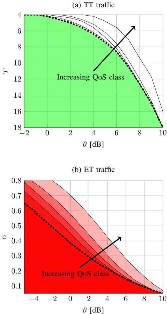
Fig. 11: Pareto frontiers between detection threshold and traffic load for  $N = 5$ . Dashed lines represent the spatially averaged frontiers.
