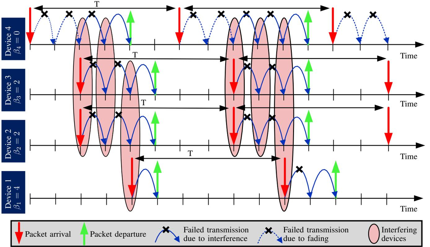
Fig. 3: Packets generation, departure process, and mutual interference between devices under TT traffic with duty cycle  $T = 6$ .
