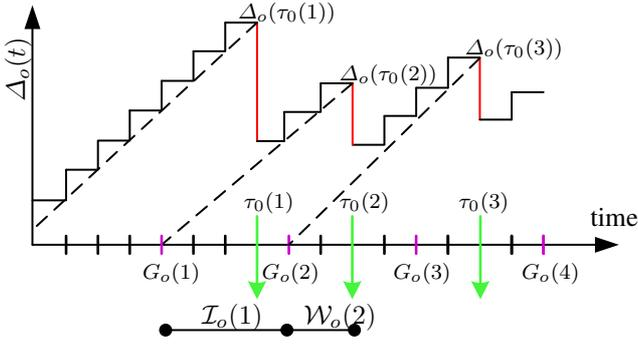
Fig. 2: AoI evolution of a typical link. The time stamps  $G_o(n)$  and  $\tau_o(n)$  denote the time at which the  $n$ -th packet was generated and successfully delivered.  $\mathcal{I}_o(1)$  and  $\mathcal{W}_o(2)$  denote the inter-arrival time and the waiting times.
