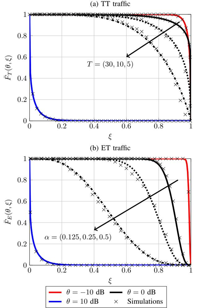
Fig. 6: Meta distribution for TT and ET traffic models.
