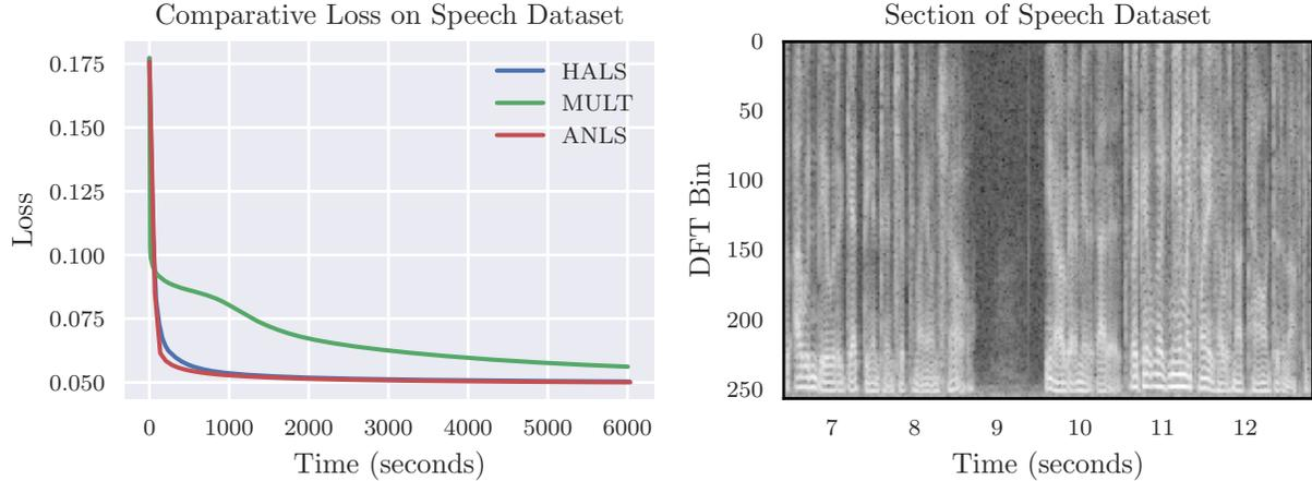
Fig. 4. Comparison of algorithms on a large speech dataset. **Left:** Normalized loss,  $\|\mathbf{X} - \hat{\mathbf{X}}\| / \|\mathbf{X}\|$ , achieved by each algorithm as a function of computation time. Both HALS and ANLS converge significantly faster than multiplicative updates. **Right:** a small slice of the speech dataset, representative of the full recording.
