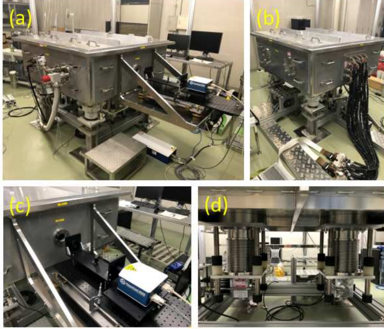
Figure 4: Picture of test system: (a) window-side view of PINOCO; (b) driver-side view of PINOCO; (c) measurement system in front of the window; (d) GM-cycle coolers
