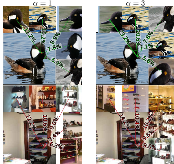
Figure 7. Influence of \alpha on the classification decisions. As in Figure 2, we visualize the most relevant corresponding image regions for the classification decision. A larger \alpha increases the importance of the most related regions in the training images. Hence the decision is based on few important regions. \alpha is set manually in this experiment.
