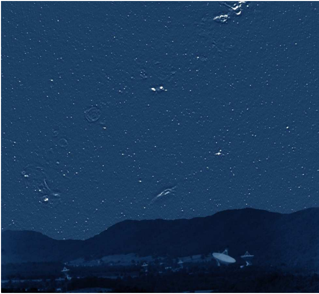
Fig. 1 The radio sky at 4.85 GHz above an optical photograph of the NRAO site in Green Bank, West Virginia (USA). The former 300-foot telescope made this image, which is about 45^\circ across. Increasing radio brightness is indicated by lighter shades to indicate how the sky would appear to someone with a “radio eye” 300 feet ( \sim 91 metres) in diameter. The flux density limit is \sim 25 mJy (Gregory et al., 1996). Copyright NRAO.
