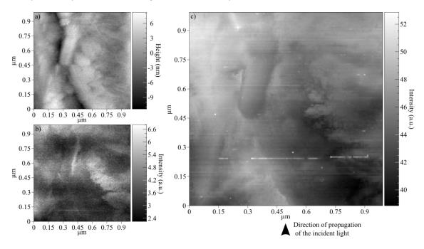
Figure 3:1  $\mu$ m × 1  $\mu$ m scanning images of the gold surface a) Topography b) Intensity of the elastically scattered light c) Intensity of the luminescence.
