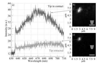
Figure 2: a) Luminescence from the apex of the gold tip. b) and c) Mapping of the luminescence intensity of the tip when it is respectively in or not in contact with the gold surface. Insets represent the tip (top) sample (bottom) configuration seen by the scanning objective.
