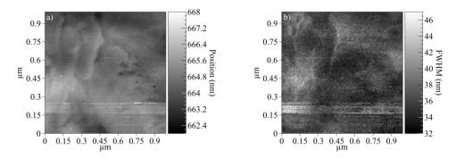
Figure 4:  $1 \mu m \times 1 \mu m$  scanning images of the gold surface. The luminescence curve is fitted with a lorentzian and the following parameters are reported a) Position of the maximum b) Full Width Half Maximum map of the fitted curve.
