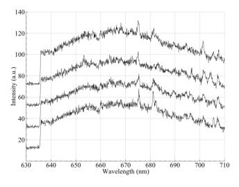
Figure 5: Luminescence for the region at  $y = 0.25 \mu m$ . Some unidentified Raman modes (sharp peaks) are clearly present. The offset between the four spectra is for clarification only.
