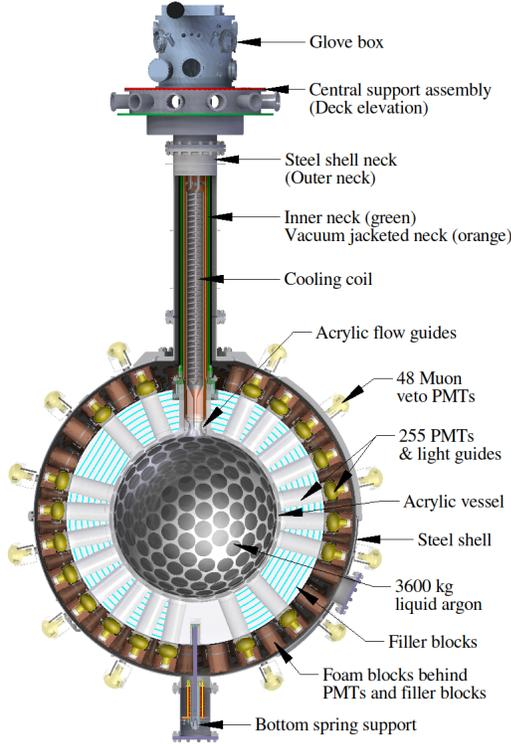
Figure 1: Central parts of the DEAP-3600 detector.
