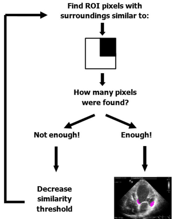
**Figure 5:** A diagram describing the search for valve corner pixels (for the left corner an “L” shaped mask is used, and its mirror image is used for the right corner)
