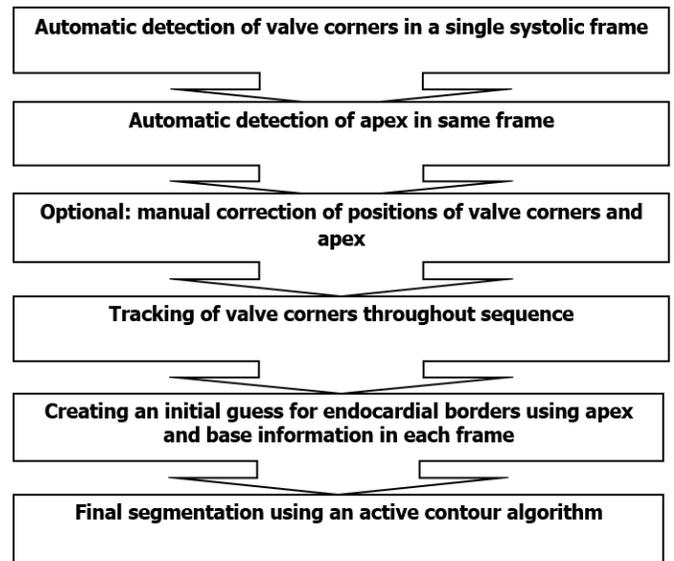
**Figure 1:** flow chart of segmentation algorithm corner-pixels per corner. The last procedure appears as a diagram in figure 5. The final corner location is the mean location of these pixels. Figure 6 exhibits an example of the corner pixels (a) and the final corner locations (b).
