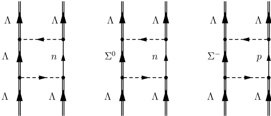
FIG. 1: Goldstone diagrams for the evaluation of the  $\Lambda\Lambda \rightarrow \Lambda n$ ,  $\Lambda\Lambda \rightarrow \Sigma^0 n$  and  $\Lambda\Lambda \rightarrow \Sigma^- p$  decay rates in infinite nuclear matter.
