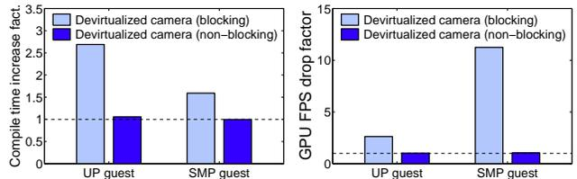
**Figure 6: Impact of a devirtualized camera at different devirtualization modes on a concurrent compile benchmark (Left), and on a concurrent devirtualized GPU (Right). The dashed line shows the no-impact value, or complete concurrency.**
