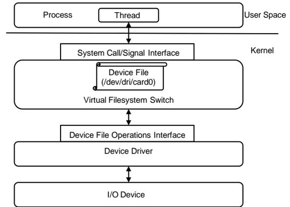
Figure 1: The simplified I/O stack in Linux
