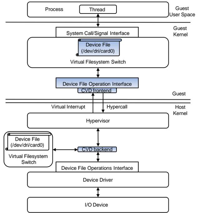
Figure 2: Devirtualization architecture
