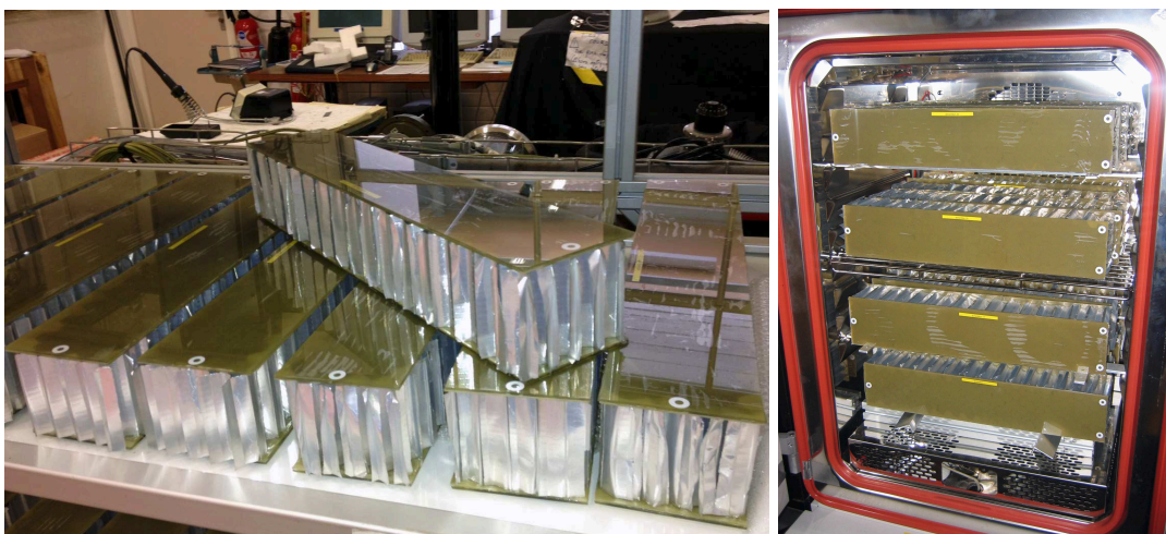
Figure 11: Left : Small samples of 100 mm by 50 mm by 80 mm with a curvature radius of 30 m. Right : Samples inside the climate chamber.
