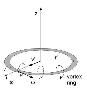
FIG. 1: Vortex ring whose radius varies with the radial velocity  $v_r$ .
