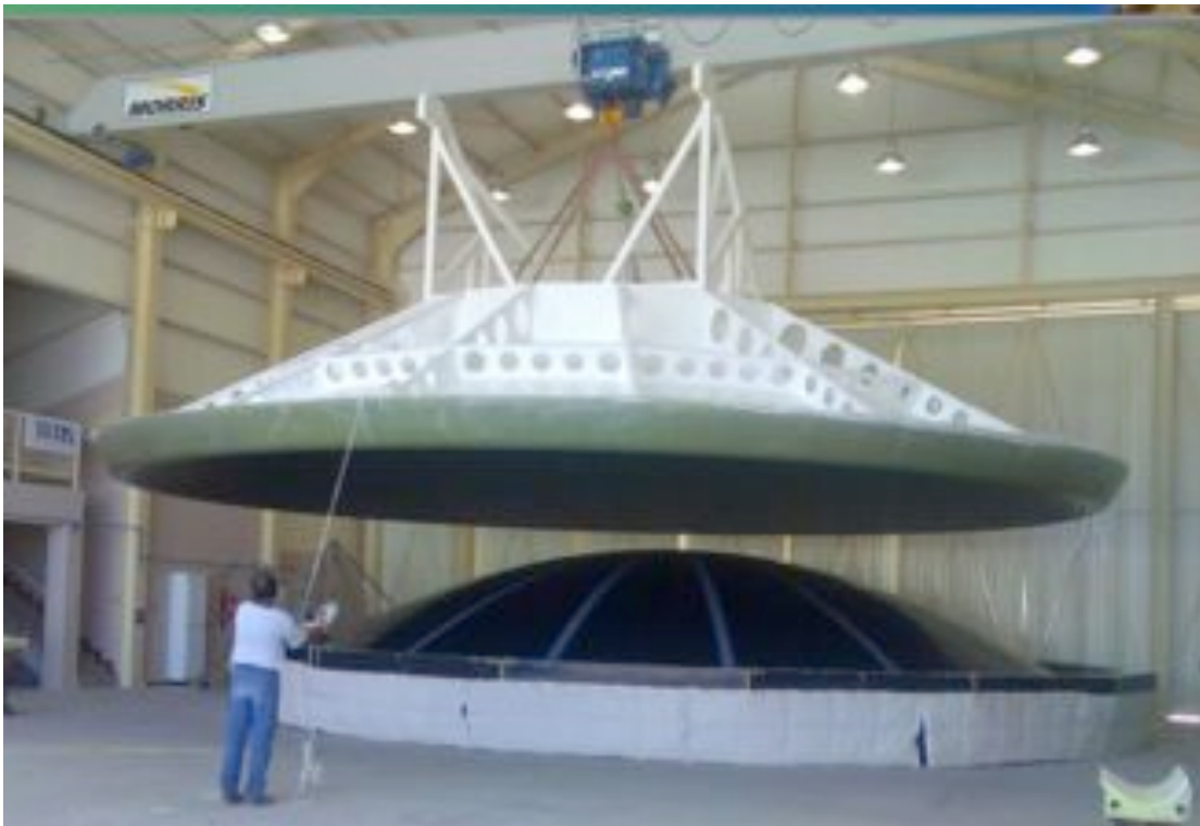
Figure 5: Research via the US SKA Technology Development Program (TDP) and direct experience via the production of composite dishes for the South African MeerKAT project, and the metal antennas of the Australian ASKAP project, indicate that a target surface accuracy of 0.5 mm (r.m.s.) or better is achievable. Image above: courtesy of the MeerKAT project.
