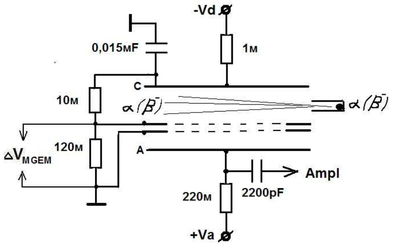
Fig.2. The chamber for MGEM tests.
