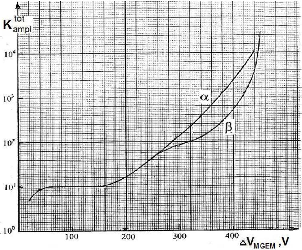
Fig.3. Dependences for the total proportional electron multiplication coefficients  $K_{ampl}^{tot}$  from the potential difference between MGEM electrodes at pressure of 1 bar and for the amplification of electrons in anode gap ( $K_{ampl}^{anode}=10$ ).
