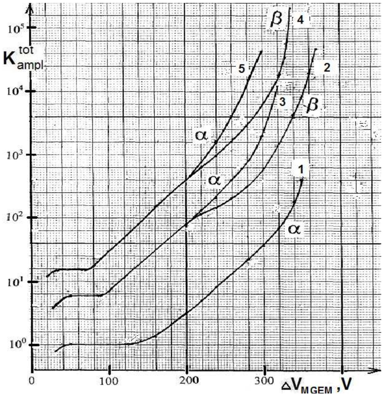
Fig.4. Dependences for the total proportional electron multiplication coefficients  $K_{\text{ampl}}^{\text{tot}}$  from the potential difference between MGEM electrodes at pressure of 0.4 bar and for the amplification of electrons in anode gap:
