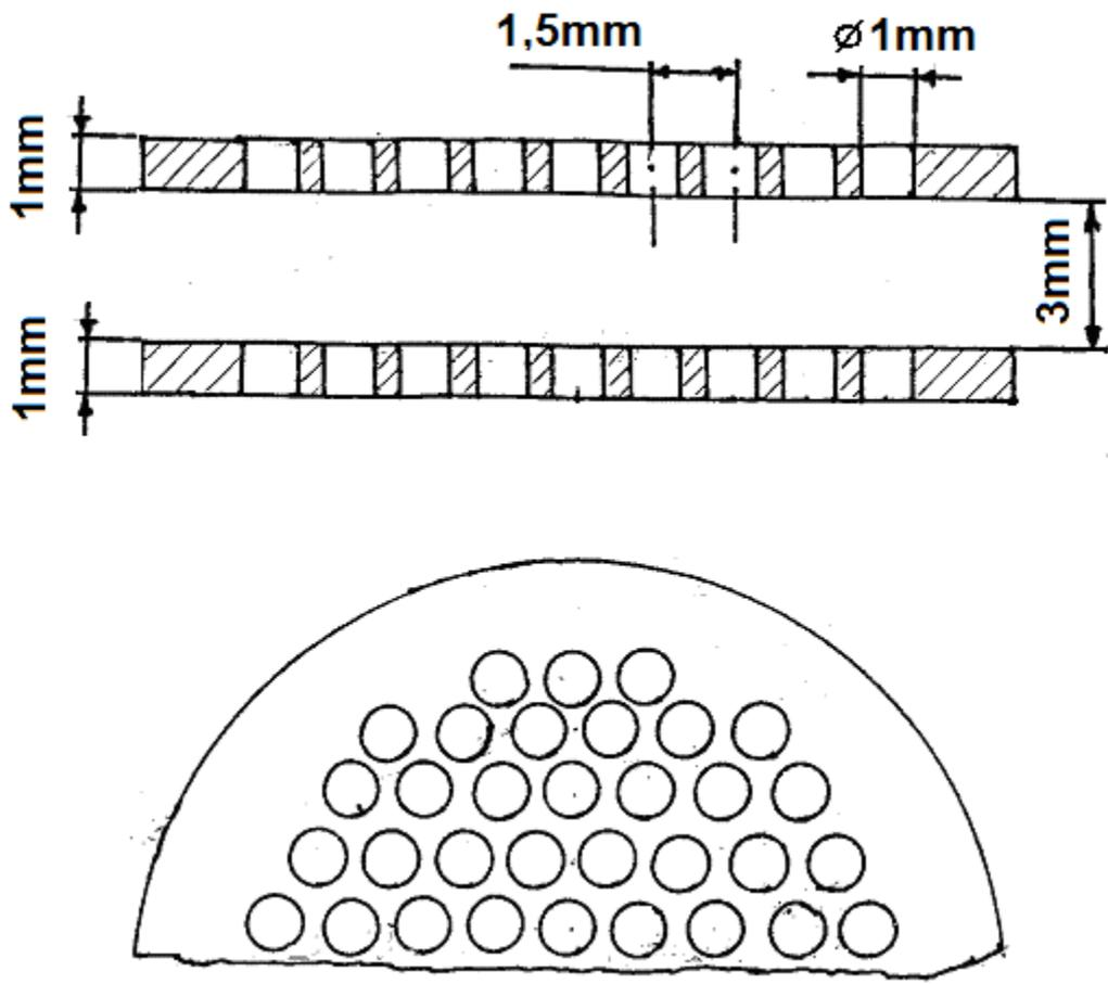
Fig.1. MGEM detector layout.
