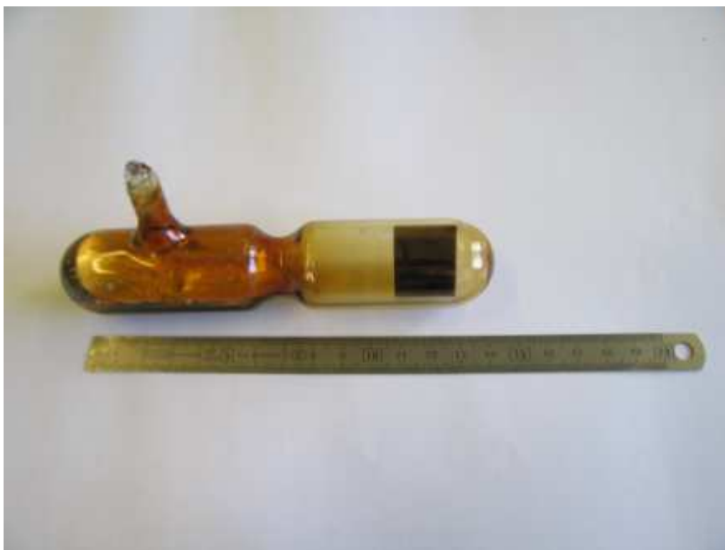
Figure 4: Typical cell made from Pyrex used for intercalation. The potassium is on the left and causes at T \geq 250 °C the brown colouring of the glass. On the right: a stage-2 intercalated graphite.
