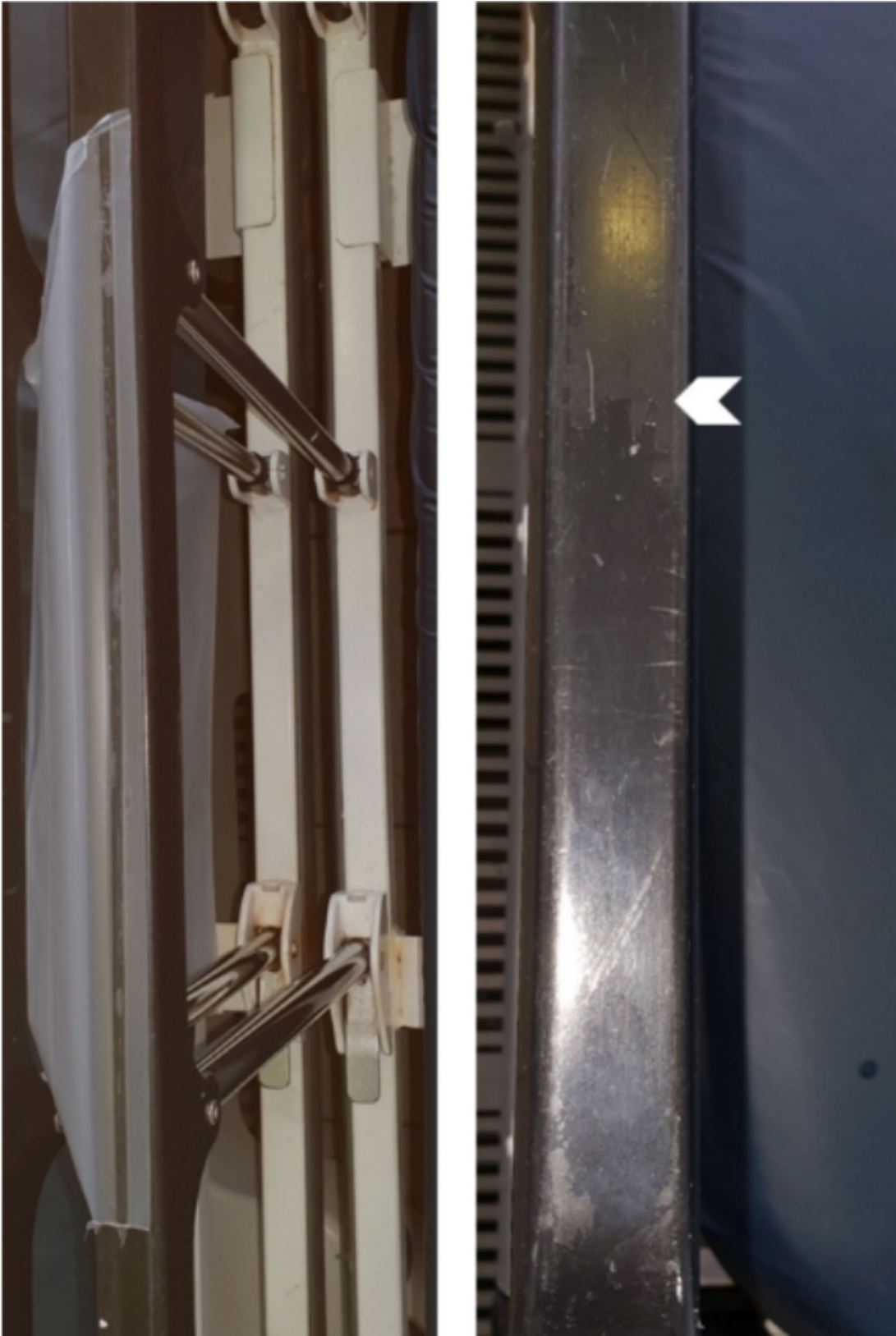
Fig. 2 (Left) Photograph of plastic bag adhered onto stretcher rail via adhesive strip. (Right) Photograph of stretcher rail with visible signs of stripped antimicrobial coating (white arrow)
