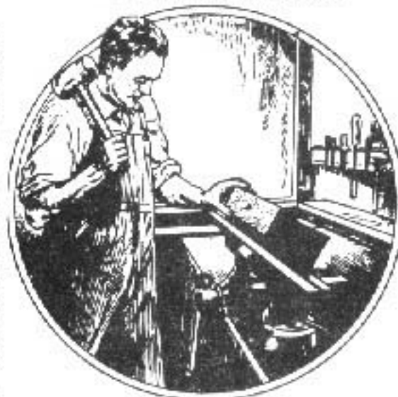
Sheet Metal Clamped in Vise Is Bent by Means of Wooden Block and Mallet
