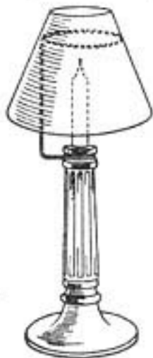
Two Forms of Shade Holder Made of Copper Wire for a Candlestick
