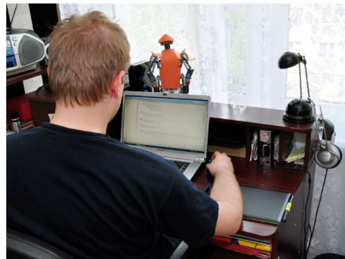
Fig. 2. The first implementation of APOEW. Note the custom clothing of the robot. APOEW is placed next to the computer screen so that interacting with the robot requires movement.
