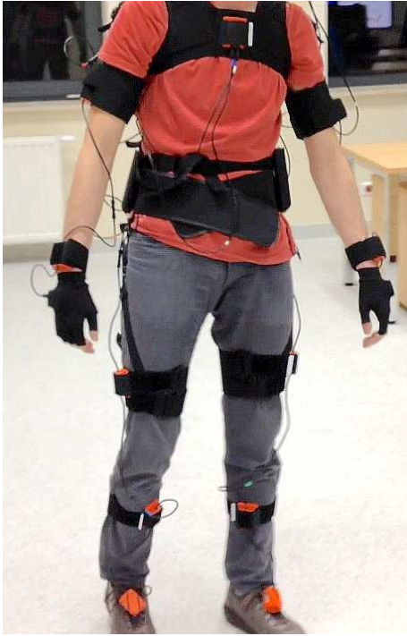
Fig. 1. Inertial sensors attached to body segments.
