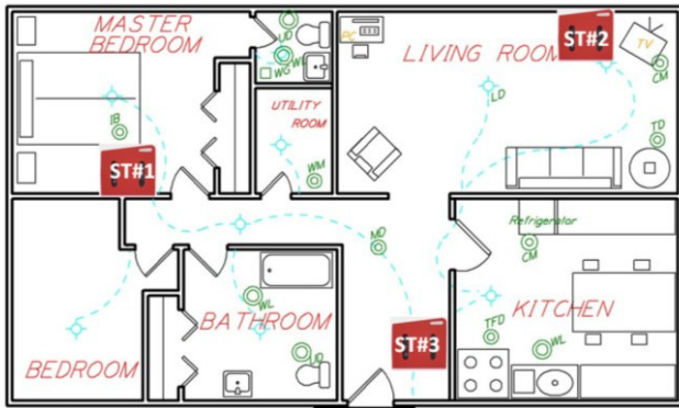
Fig. 7 Example of possible implementation in home environment for three TI CC2650 SensorTags
