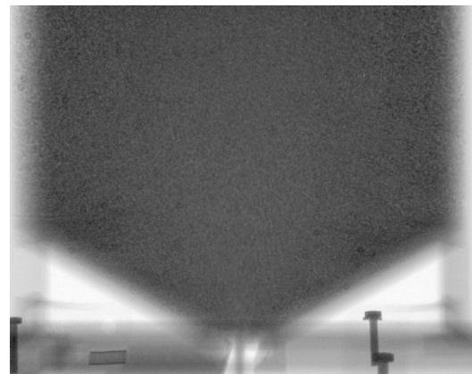
Fig. 4. Radiography image with free granular flow
