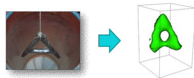
Fig. 1. Object and 3D reconstruction obtained using Electrical Capacitance Tomography
