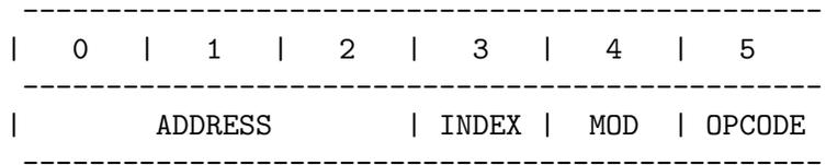
For a given instruction, ‘M’ stands for the memory address obtained after indexing the ADDRESS subfield (using its INDEX byte), and ‘V’ is the contents of the subfield indicated by MOD of the memory cell with address ‘M’. For instance, suppose that we have the following contents of MIX registers and memory cells:
