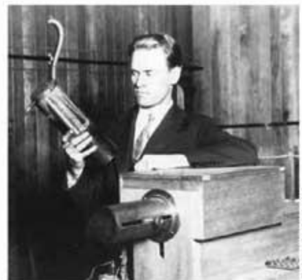
Figure 3: Philo Farnsworth holds an image dissector used in his early television camera
