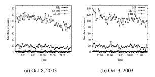
Figure 6. Comparing multi-resolution and single-resolution detection
