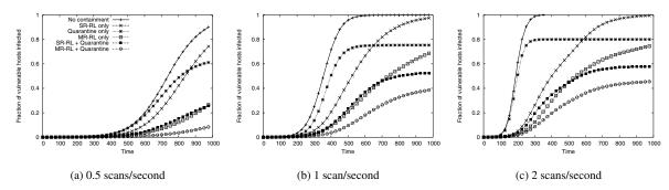
Figure 9. Comparing different containment mechanisms for various worm scanning rates
