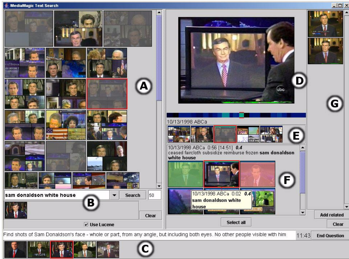
Figure 2: The interactive search interface. (A) Story keyframe summaries in the search results (B) Search text and image entry (C) TRECVID topic display (D) Media player and keyframe zoom (E) Story timeline (F) Shot keyframes (G) Relevant shot list
