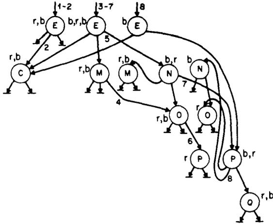
FIG. 10. A partially persistent red-black tree built using the node copying method of Section 2. The sequence of operations consists of insertions of  $E$ ,  $C$ ,  $M$ ,  $O$ ,  $N$ ,  $P$ ,  $Q$ , followed by deletion of  $M$ . Extra pointers are labeled with their version stamps. Each node is labeled with its successive colors. Insertion of item  $N$  triggers the transformation in Fig. 8d. Deletion of  $M$  triggers the transformation in Fig. 9d.
