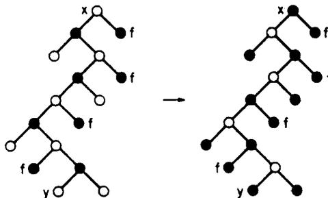
FIG. 11. An insertion interval with top node  $x$  and bottom node  $y$ , showing the desired recoloring. The nodes marked “ $f$ ” are the fringe nodes of the interval. The interval is represented by storing in node  $x$  the item in node  $y$  (which is also still stored in  $y$ ) along with a flag indicating that  $x$  is the top of an insertion interval.
