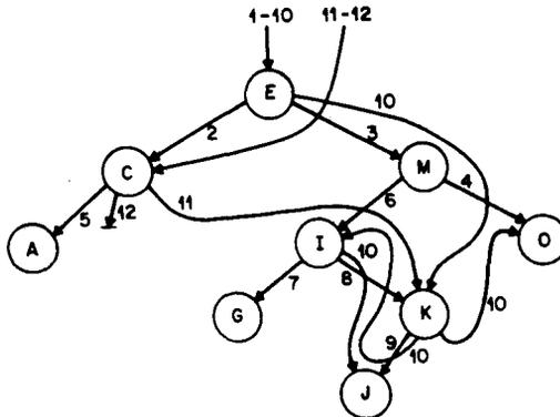
FIG. 1. A partially persistent search tree built using the fat node method, for the sequence of update operations consisting of insertions of  $E$ ,  $C$ ,  $M$ ,  $O$ ,  $A$ ,  $I$ ,  $G$ ,  $K$ ,  $J$ , followed by deletion of  $M$ ,  $E$ , and  $A$ . The "extra" pointers are labeled with their version stamps. Left pointers leave the left sides of nodes and right pointers leave the right sides. The version stamps and original null pointers of nodes are omitted, since they are unnecessary.
