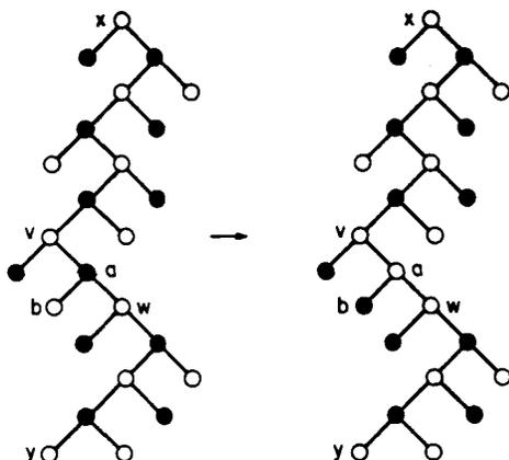
FIG. 13. Splitting an insertion interval. The nodes in the interval have their uncorrected colors. Recoloring the nodes  $a$  and  $b$  splits the insertion interval from  $x$  to  $y$  into two insertion intervals, one from  $x$  to  $v$  and one from  $w$  to  $y$ .
