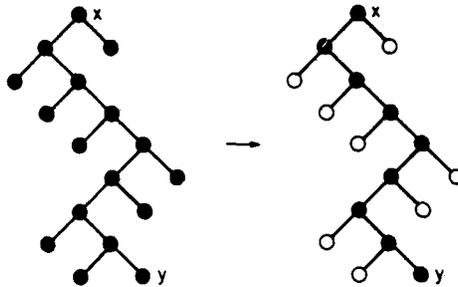
FIG. 12. A deletion interval with top node  $x$  and bottom node  $y$ , showing the desired recoloring. The interval is represented by storing in node  $x$  the item in node  $y$  along with a flag indicating that  $x$  is the top of a deletion interval.
