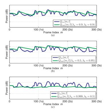
Fig. 4. Sample inputs (solid curves) and outputs (dashed curves) of the asymmetric nonlinear filter defined by Eq. (4) for conditions when (a)  $\lambda_a = \lambda_b$  (b)  $\lambda_a < \lambda_b$ , and (c)  $\lambda_a > \lambda_b$ . In this example, the channel index l is 8.
