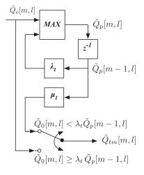
Fig. 5. Block diagram of the components that accomplish temporal masking in Fig. 3.
