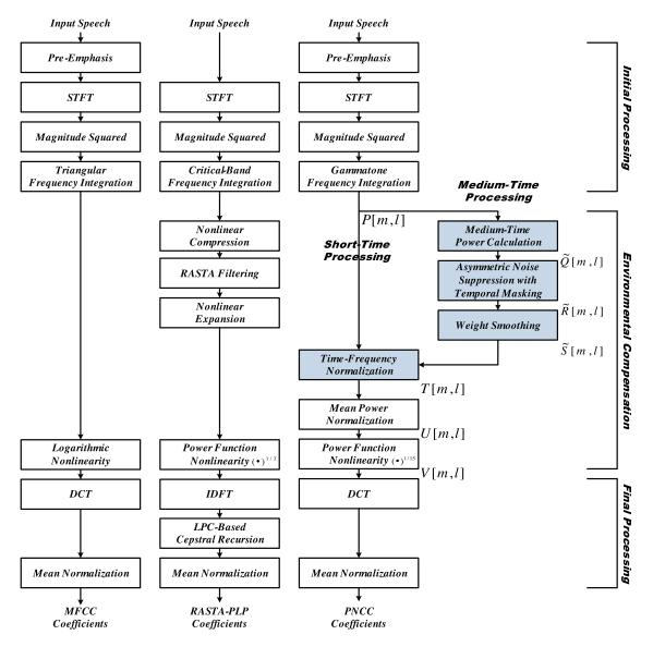
Fig. 1. Comparison of the structure of the MFCC, PLP, and PNCC feature extraction algorithms. The modules of PNCC that function on the basis of "mediumtime" analysis (with a temporal window of 65.6 ms) are plotted in the rightmost column. If the shaded blocks of PNCC are omitted, the remaining processing is referred to as *simple power-normalized cepstral coefficients (SPNCC)*.
