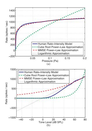
Fig. 9. Comparison between a human rate-intensity relation using the auditory model developed by Heinz *et al.* [64], a cube root power-law approximation, an MMSE power-law approximation, and a logarithmic function approximation. Upper panel: Comparison using the pressure (Pa) as the *x*-axis. Lower panel: Comparison using the sound pressure level (SPL) in dB as the *x*-axis.
