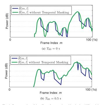
Fig. 6. Demonstration of the effect of temporal masking in the ANS module for (a) clean speech, and (b) speech in simulated reverberation  $T_{60} = 0.5$  s. In this example, the channel index *l* is 18.
